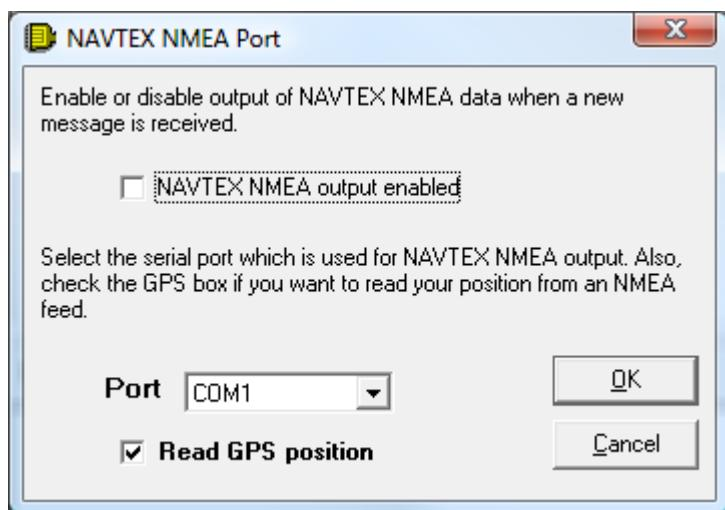
Tick the box Read GPS Position if you have a GPS connected, and select the COM port. NAVTEX NMEA output enabled sends NAVTEX alarm settings out, for example to parts of an ECDIS system. In most installations it is unticked.
