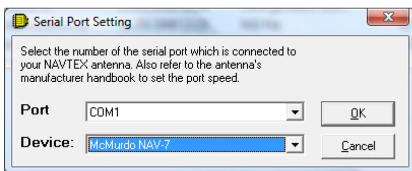
Now select the COM port (all available COM ports are listed in the drop-down box), and the make and model of your NAVTEX receiver. Then click on the Start button on the toolbar, and Navtex messages will be received.
