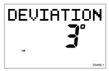
This shows the maximum deviation detected, and indicates that compass correction has been completed successfully.
