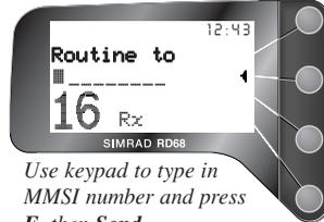
Use keypad to type in MMSI number and press **E**, then **Send**
