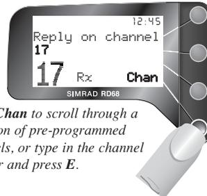
Press **Chan** to scroll through a selection of pre-programmed channels, or type in the channel number and press **E**.
