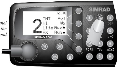
If channel selection is not confirmed within 2 seconds (by pressing E), the radio will revert to the original channel
