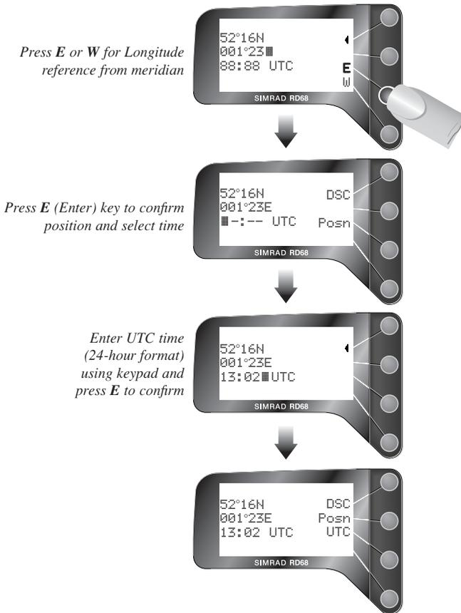
**Note** *The display will now show the manual Lat and Long when in DSC mode, but the clock display will not be shown (this is only available if NMEA position and time data is being received).*
