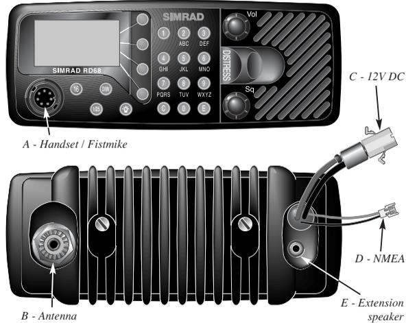
Fig 4.4 - External connections
