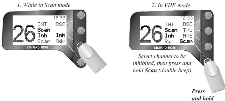
To re-enable an inhibited channel into the scan cycle, repeat sequence 2:
