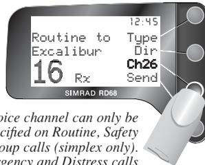
Voice channel can only be specified on Routine, Safety and Group calls (simplex only). Urgency and Distress calls are set to Ch16. When making a Routine call to a coast station (MMSI begins with "00"), the option to select a voice channel is not available.
