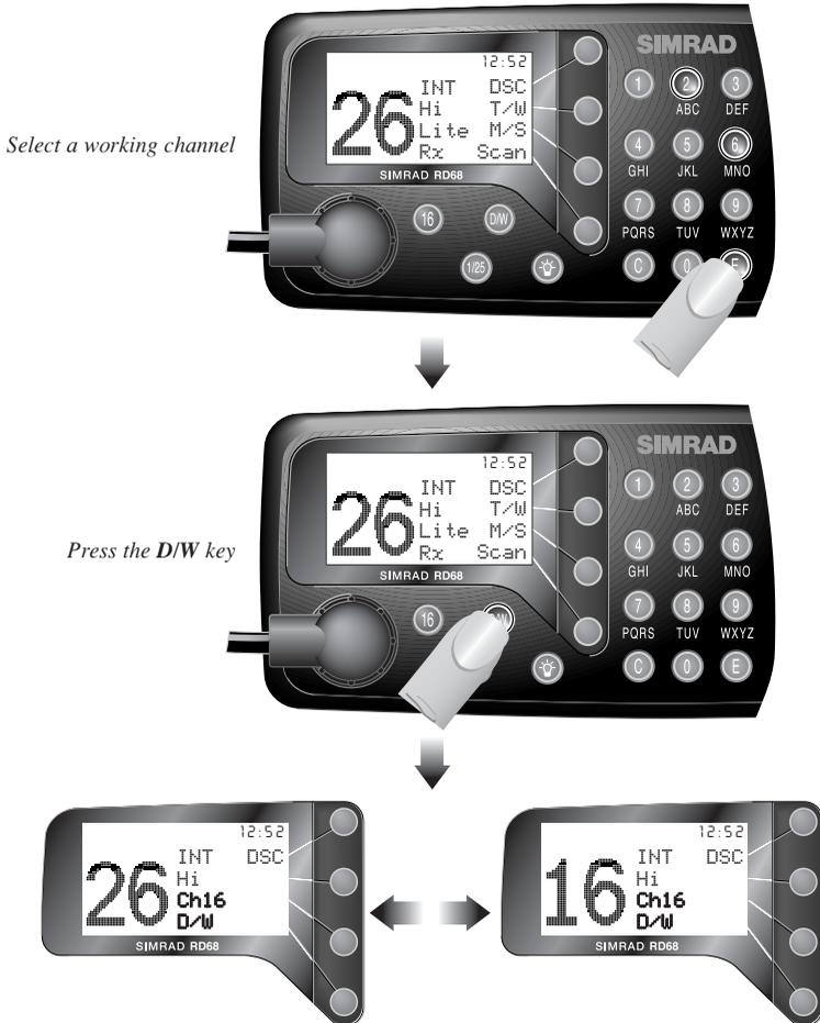
The RD68 will monitor the working channel and the priority channel sequentially
