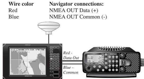
Fig 4.5 - Linking to navigation source
